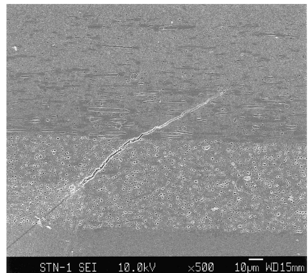
Fig. 5. Crack deflection at the layer interface.
